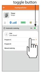
(3) You can set a start time, duration (from 1 minute to 3 hours and 59 minutes) and the days of the week you want to irrigate on for each programme. If you want the programme set to be operational immediately, make sure that the toggle button is on. Press the Save key and return to confirm the settings.
